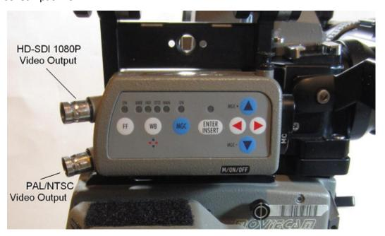
The upper BNC connector is SDI digital video output. The lower BNC and 4-pin Fischer connectors are analog video outputs. You can get HD analog video signal in AHD, TVI or CVI formats by setting these formats on ANALOG MODE from SYSTEM/OUTPUT. For a regular SD analog PAL/NTSC monitor only analog CVBS format will work.
