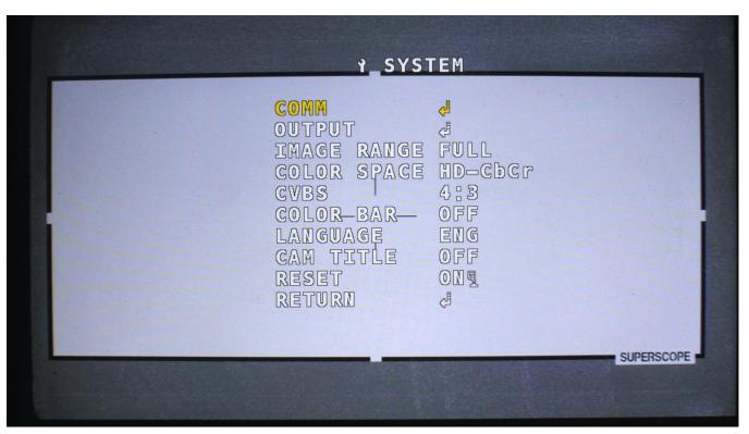
By keeping the **4:3 CVBS** frame ratio for SD PAL/NTSC signal and setting the ratio at 16:9 on the SD monitor the frame will be similar to that one on the HD monitor.
