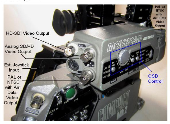
The upper left BNC connector is SDI digital video output. The lower BNC and 4-pin Fischer connectors are analog PAL or NTSC video outputs with Arri data. The upper right BNC connector is analog: SD-PAL/NTSC or HD video output in AHD, TVI or CVI formats. You can set the analog HD formats from OSD MENU SYSTEM/OUTPUT/ANALOG MODE. For a regular SD analog PAL/NTSC monitor only CVBS analog mode will work.
