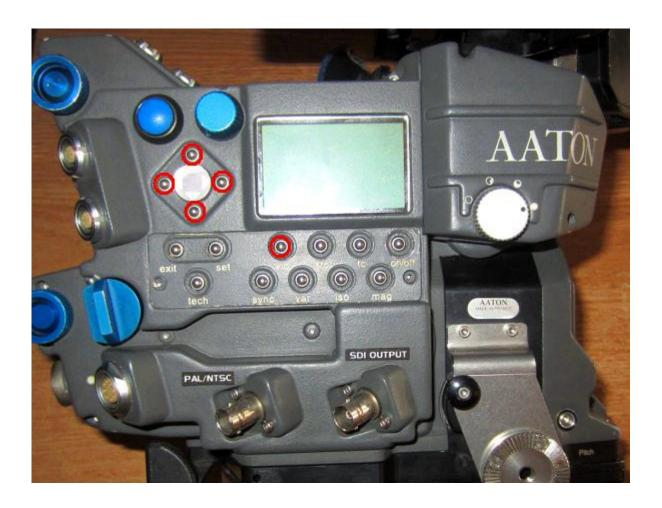
The right BNC connector is HD SDI digital video output: 3G-SDI (SMPTE424M Compliant) 1080P60/50, HD-SDI (SMPTE292M Compliant) 1080P30/25, 720P60/50, 720P30/25. The left BNC and upper 4-pin Fischer connectors are analog SD PAL/NTSC (CVBS) video outputs or HD analog video outputs in AHD, TVI or CVI formats. The lower 4-pin Fischer connector is 12V DC output only.
