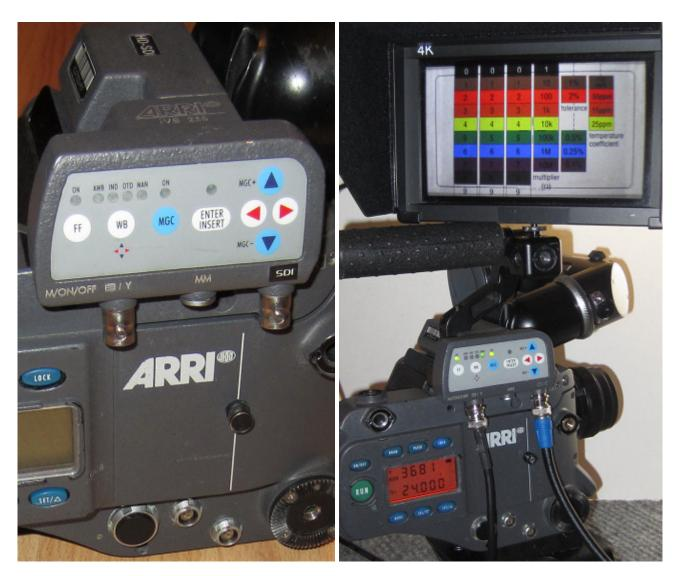
The converted IVS unit produces a near flicker-free image for a camera speed of 24fps, and a flicker-free image for camera speeds of 25fps and 30fps. It has two video outputs:
