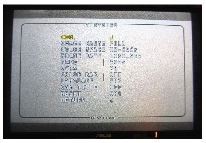
The SYSTEM/RESET function clears the current MENU setting and introduces the default setting in which the HD system will automatically change the setting to 60Hz and SD to NTSC.
