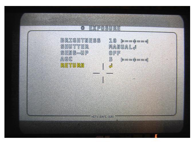
In very low light, you can switch SHUTTER to AUTO and set the X2 - double exposure image.
